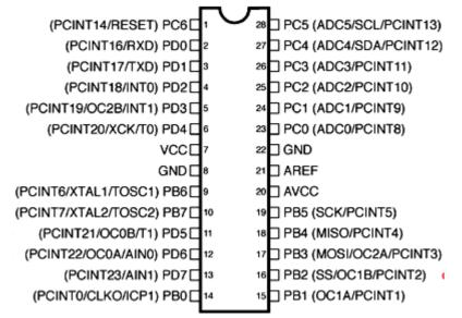
Figure 1: Pin diagram of ArduinoUNO
